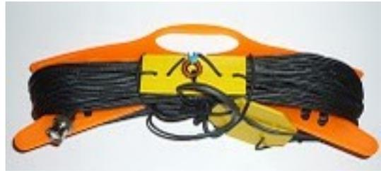
The center insulator and insulator under the trap is CNC made from plastic plate. The center insulator has a hole with 7mm diameter, which serves to plug the fiberglass whip. Design of center insulator is evident from the figure, the fixing is made from cable ties and heat-shrinkable tubing.
